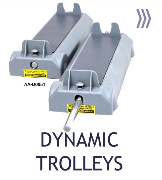
An affordable and effective teaching aid for demonstration in potential / Kinetic Theories. With features that allow additional weights to be loaded, experiments in velocity, acceleration and collision can be conducted with ease. A teaching apparatus to explore Newton's Laws
