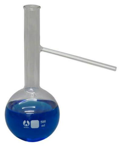
Long neck borosilicate glass flask comes with a distilling arm (stem). Distillation is a widely used method for separating mixtures based on differences in the conditions required to change the phase of components of the mixture. To separate a mixture of liquids, the liquid can be heated to force components, which have different boiling points, into the gas phase. The gas is then condensed back into liquid form and collected
