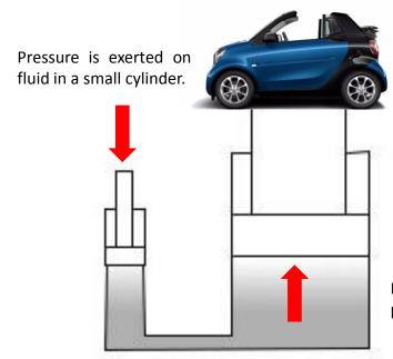
Though the pressure is the same, it is exerted over a much larger area, giving a multiplication of force that lifts the car.
