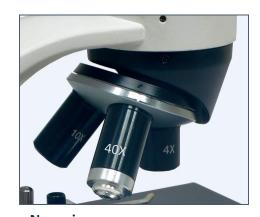
**Nosepiece** Trinocular nosepiece with precise click stop, Equipped
