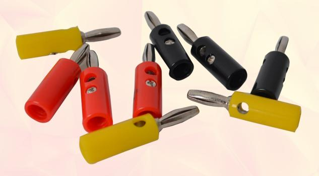
The 4 mm pin has a spring insert and the rear of the plug has a 4 mm socket. The wire is attached by means of a clamping screw in the bottom of the socket. Maximum current carrying capacity : 10 A
