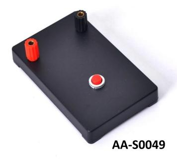
Push-on button type, made of plastic material, attached to a plastic base with 4mm socket terminals (spin-free).
