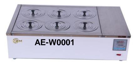
Water bath is a laboratory equipment used to incubate samples in water at a constant temperature. Our water bath come with stainless steel interior chamber and epoxy-coated cold rolled steel board exterior which make them resistant to corrosion and chemical damage.
